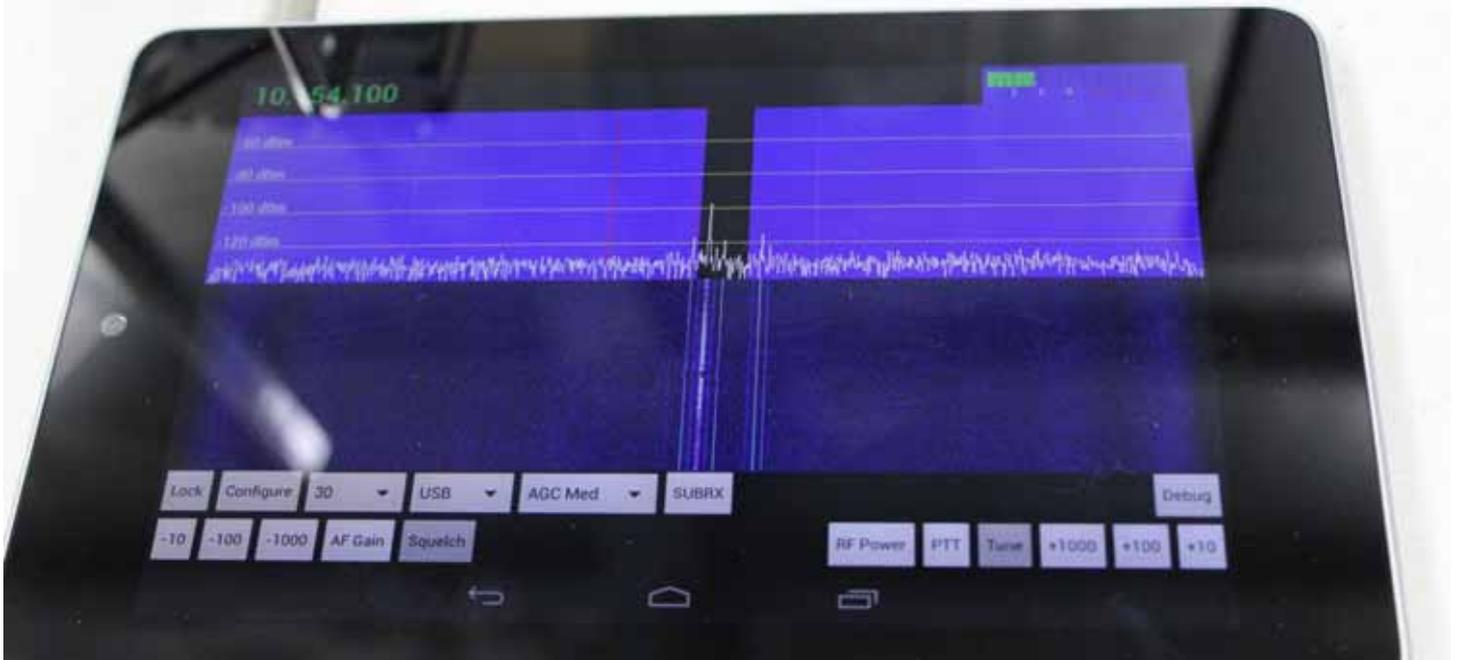
SDR on an Android Tablet, the table is the PC; all connected wirelessly, SDR transceiver in the palm of your hand...
