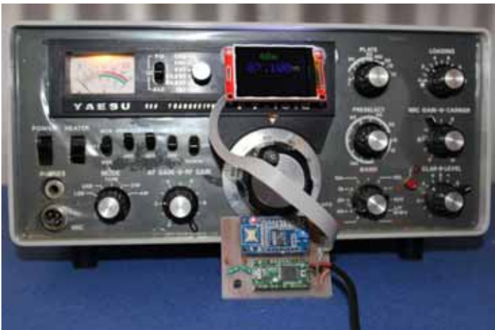
FT101E with added digital readout ↑
