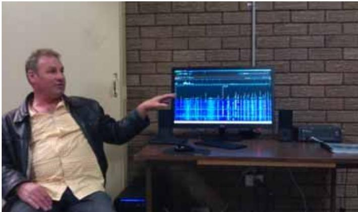
Don explains the amazing capability of HPSDR ↑ Only using about 6% of the computers processing power, its possible to "watch" via a waterfall display, in real time, from the AM broadcast band right up to 6 meters.
