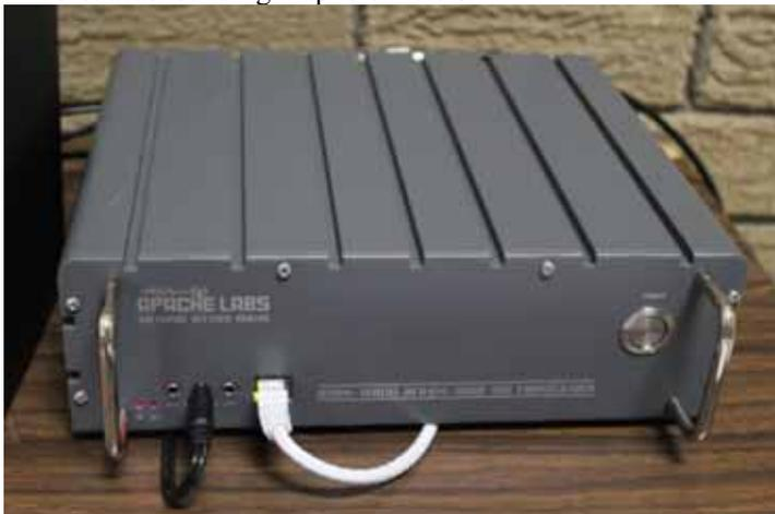
A complete 100 watt SDR Transceiver, HF to 6 meters. ↑ Even with a wire inverted 'V' right under the EHT powerlines outside in the car park, virtually no interference was heard due to the superior noise processing power of the SDR software within the computer. No computer or noise from the switch mode supply under the table either - this is a real DX'ers tool...
