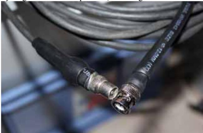
The existing 'N' connectors on the ATV RX beams were replaced with twist on/off BNC connectors. With summer and daylight savings soon, time to get ready for some portable operations. ~Mick VK3CH
