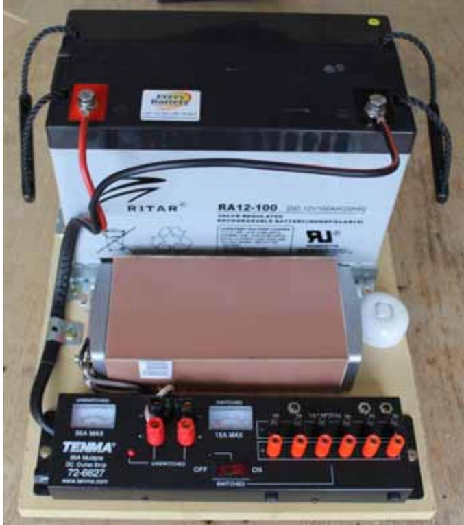
The distribution board Don VK3HDX found on EBay new, just \$60, Tough and well made. You couldn't make this for \$60! To feed the camera and portable TV, Mick added some DC plugs to the distribution block. The DC board inside. ↓
