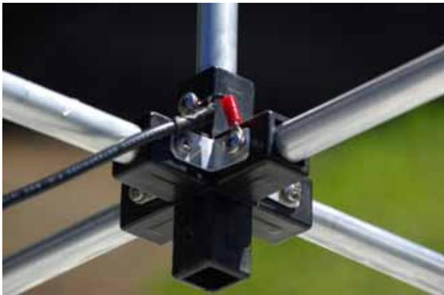
← Showing coax connected to the ground plane and to the driven element. Also the aluminium angle shorting strips interconnecting the ground plane.
