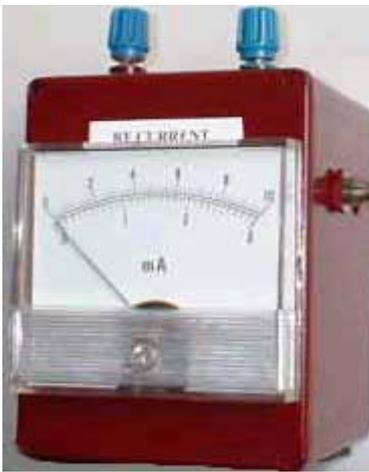
To the left is a picture of the offending RF ammeter. The two terminals on the top are connected together inside the box with heavy wire which runs through the centre of a toroid, making the current transformer. The beauty of this arrangement is that you can stick the meter in the aerial wire or the earth connection. In fact, you can stick it anywhere you like, within reason! Click on the picture for the circuit and construction details.
