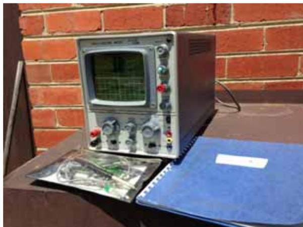
Alan VK3SM, has a BWD 509B Oscilloscope for sale. 5 inch single beam Serial No. 20650, complete with spare tube, external probes and original handbook. Bandwidth DC or 2 Hz to 7 MHz. Rise time 50n Sec over 4cm. Horizontal amplifier DC to 1 MHz. Time range 1 $\mu$  Sec to 0.1 Sec in 6 steps, Calibration <5% Triggering Internal Auto 1 cm deflection 5 Hz to 10 MHz All or any offers considered, the unit will be brought for viewing at the club March meeting (AGM) Contact Allan 9386 4406.
