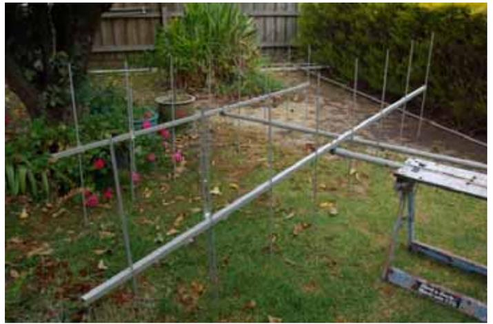
Continuing saga these are 2 meter 8 element yagi's on 3 meter booms
