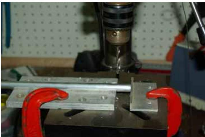
A rough drill jig to drill all of the mounting holes ↑
