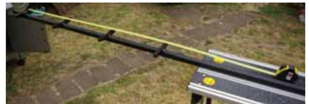
Measuring the spacing on the 2mm square boom ↑
