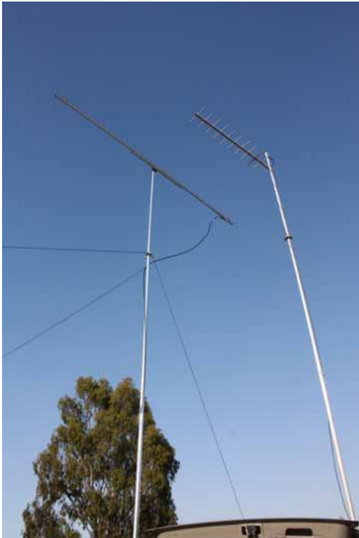
ATV 23cm TX beam and 70cm RX beams facing Mt Dandenong Improvements to VK3RTV made for perfect copy into VK3RTV2, Without any dropouts, not bad going into rear of the RX beam...
