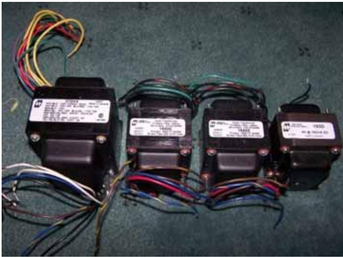
Brand new transformers, Power, 2x Output's and a Choke ↑
