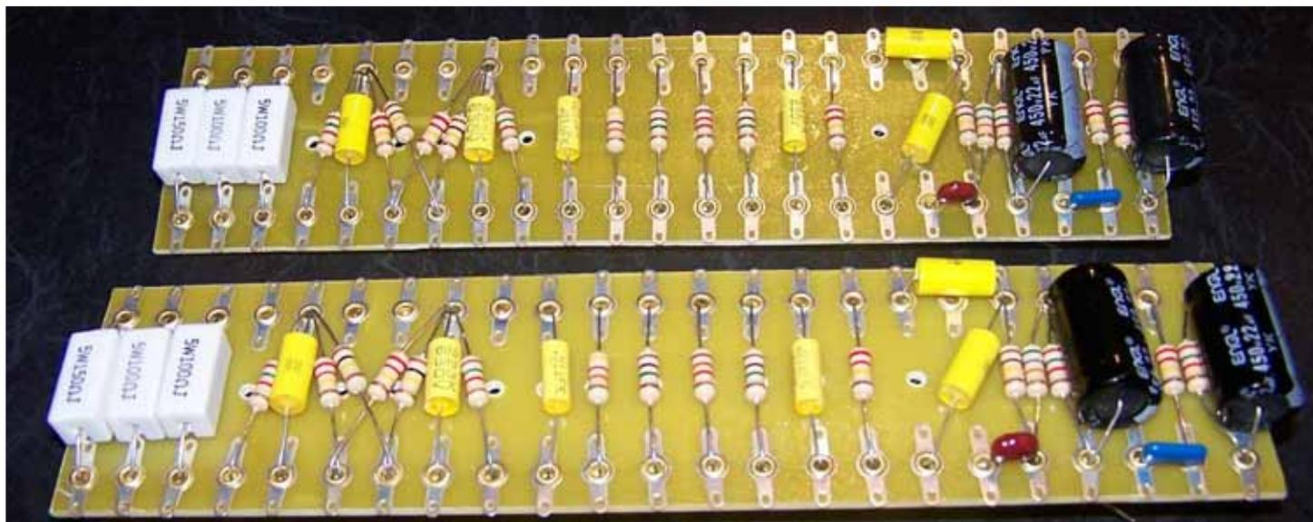
Tag Strip with components for Left & Right audio channels ready to solder up for point to point wiring ↑
