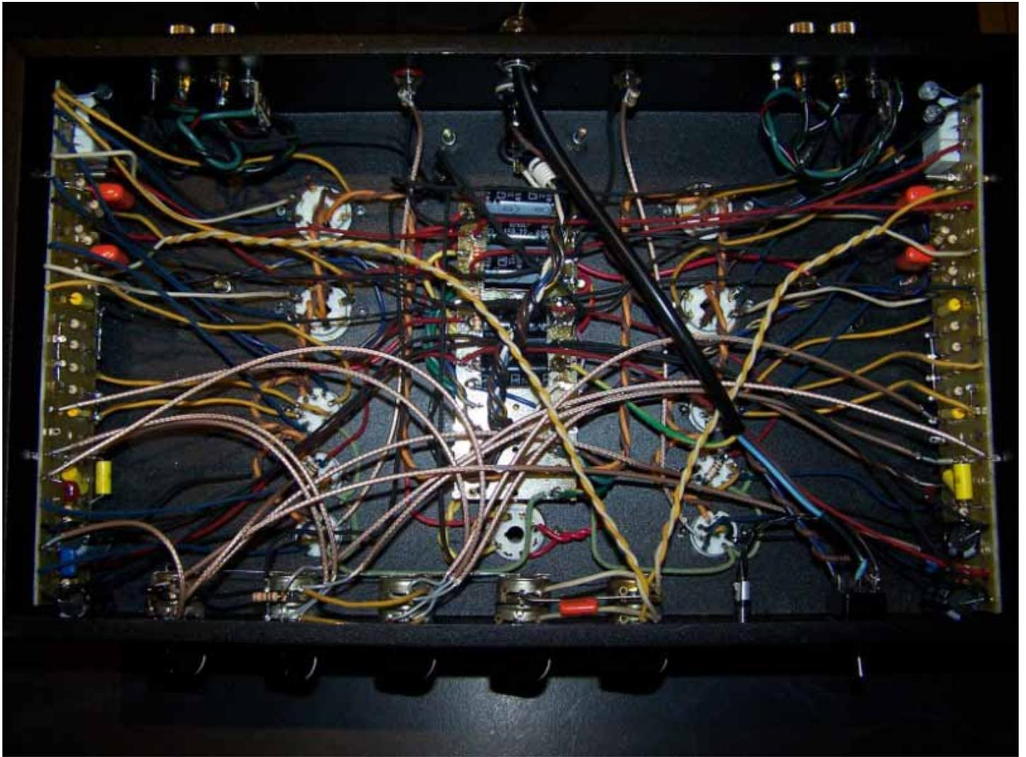
The wiring all done; Teflon coax the only 'advanced' signal carrier in the unit ↑
