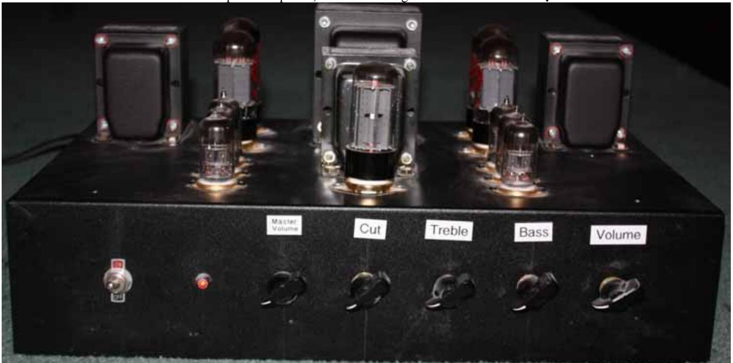
Centre valve is 5Y3GT rectifier with Choke and Power Transformer behind it.
