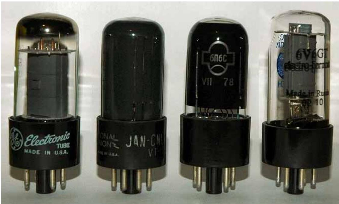
Various 6V6's manufactured around the world; from left to right; 6V6GTA by General Electric, 6V6GT JAN National Union (1940s), 6P6S (USSR, 1978) and modern production 6V6GT by Electro-Harmonix, which I used in my amplifier.
