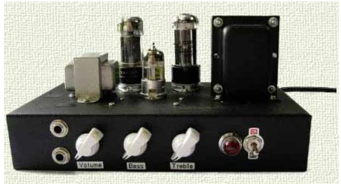
By 1955 Fender started putting its amps in the "Narrow Panel" tweed cabinet with a plastic oxblood color grill cloth, and by this time the Champ was officially named the Champ (model 5E1). Through 1957, Champs only had a six inch speaker, but the 1958 model 5F1 featured an 8". The 5E1 and 5F1 circuits used a 12AX7 dual triode in the preamplifier to provide two stages of voltage amplification, and a single 6V6GT power tube to produce about 5 watts.
