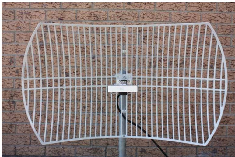
Other specs quoted are; 60MHz bandwidth, 18 degree V beamwidth, 28 degree H beamwidth, >25dB F/B ratio, 1:1.5 VSWR, 50Ω, 100 watts max input power, Dimensions 0.6m x 0.9m, 4.5kg weight, Rated wind velocity m/sec 60, mast mount diameter 40~50mm
