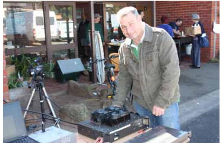
*Top beam is 23cm ATV TX mini beam, lower one 446.500MHz RX beam*
