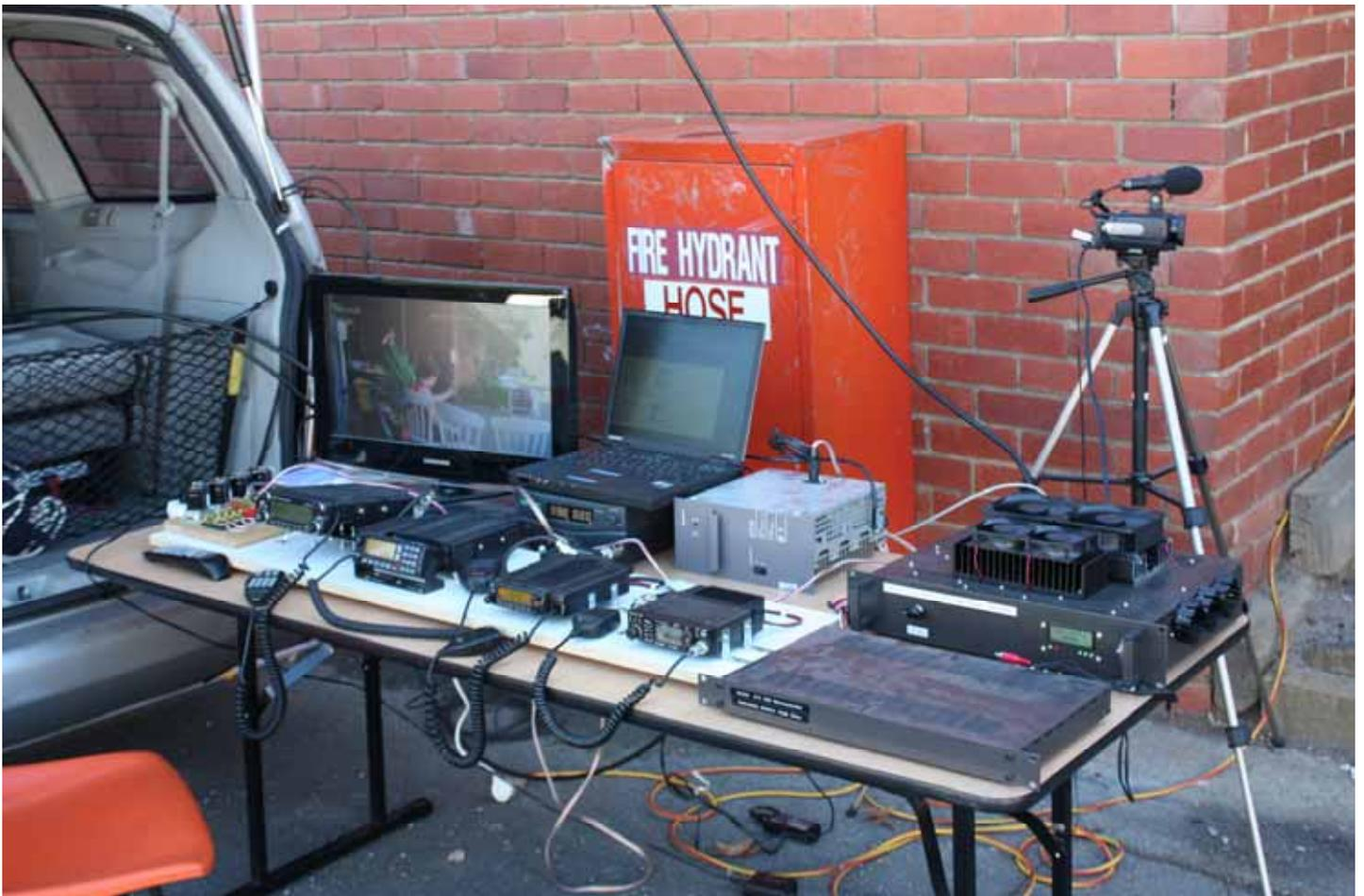
*The setup with FM voice radios at front, On-Screen Display front right; TV with laptop to program DVB-S & On-Screen Display box, two power supplies one 13.8 volts and 24 volts and the 150 watt ATV TX box at far rear right, with camera on the tripod stand. Running at full power the PA units did not get hot at all, even with the fans only spinning at half speed. During the day a VSWR meter was placed in line and the VSWR was found to be 4:1, no way an ideal match, being a loss of 36.0%.*
