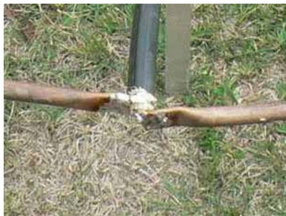
One end of the copper tube to the shield and other to the center of the coax.
