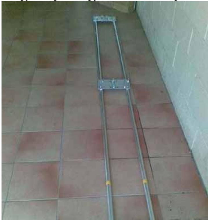
I put some yellow tape so I can know I'm near centre as I drive the car over the tubes. A plate was put in the centre to stop any spreading with car on them. The weight of the car keeps everything firm with little 'play' in the masts. Two of these give 4 masts, so I have dual X7000 antennae for VHF / UHF and another 2 for ATV TX & RX beams. It's quite light as well. If your car is smaller than you just cut the length to suit its width which will make for a more compact length for transport.
