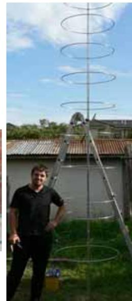
Stage three - fitted the support strut across the top of all the elements to stop them bouncing around and build the mesh reflector and off into the field to test it.
