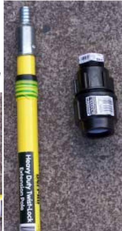
It just so happens that the tapered end fits snugly over the cast end of the extension pole. (A wrap or two of tape will hopefully make a non-slip fit)
