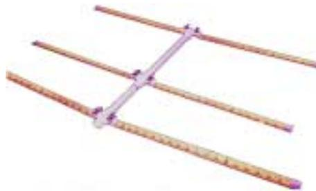
When I designed this antenna I had one basic idea in mind. It had to be easy to get in and out of the car when hunting for a hidden transmitter. This would be accomplished by the use of steel "tape measure" elements. These elements could fold easily when fitting the antenna into my car and yet still be self supporting. I decided to use three elements to keep the boom from getting too long.
