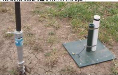
The stand on the right just sits on a reasonably flat surface and I've used some metal thread screws and wing nuts to attach a series of wire radials around the edge of the steel base plate and attached a suitably sized piece of PVC tubing using a couple of large worm-drive clamps to support the Squid-Pole. These stands are very expensive at \$70 and up, and come in both square & circular base designs. I was lucky and found my square version at one of the charity shops at \$10
