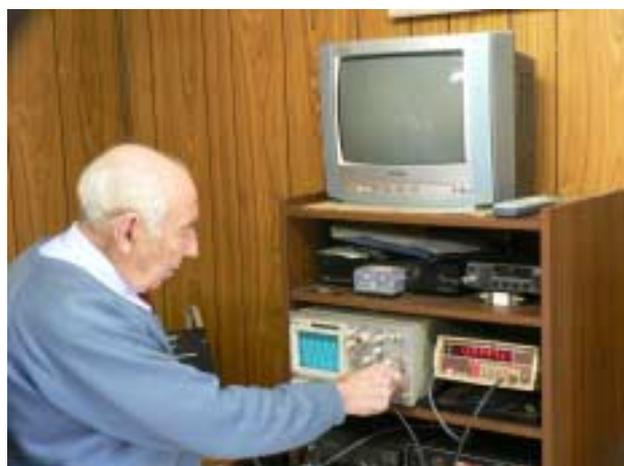
The radio required an alignment of 60.00000MHz—the top photograph shows the frequency meter and radio.
