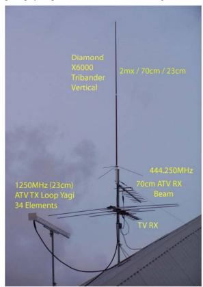
An antenna for 23cm TX & 70cm RX were roof mounted and Ian, VK3IV had his first ATV test transmission. Some adjustments to the camera were needed due to strong light, but all is progressing well. Being a HF operator in the main, the cross to the microwave bands has been quite different, but is something that he can get away with, even with antenna height restrictions on the property. But watch out - his roof might slowly end up like mine - hi!
