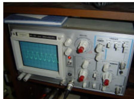
Bill VK3KBL has been busy making up an external 4MHz oscillator for the ATV PLL unit, photos show L-R, top view, bottom etched view and a nice 4MHz pattern appearing on the CRO. See page 2.
