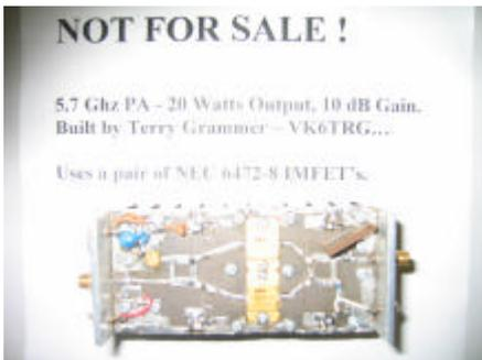
5.7GHz 20 watts Linear Amplifier
