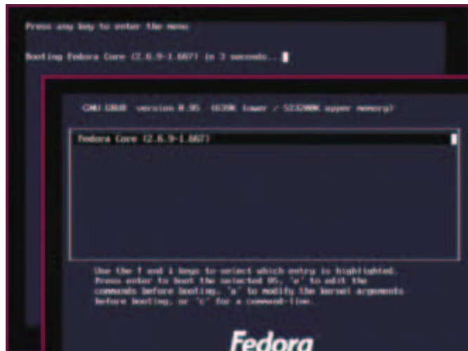
GRUB (Linux) dual boot screen with a boot option to Linux shown.
